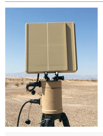
The man-portable Ranger® R6SS electronically-scanned, mid-range radars detect and track personnel and vehicles up to 15 kilometer ranges. Light and small, the Ranger R6SS provides best-in-class target detection and acquisition performance in a form factor that fits in a backpack or is easily mounted to a vehicle or permanent structure as part of an integrated solution. The low false alarm rate and extremely reliable operation builds operator trust and yields high operational availability.
