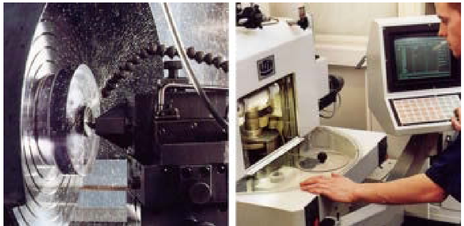
Figure 21.5 LEFT: Diamond turning machine; RIGHT: Lens polishing
