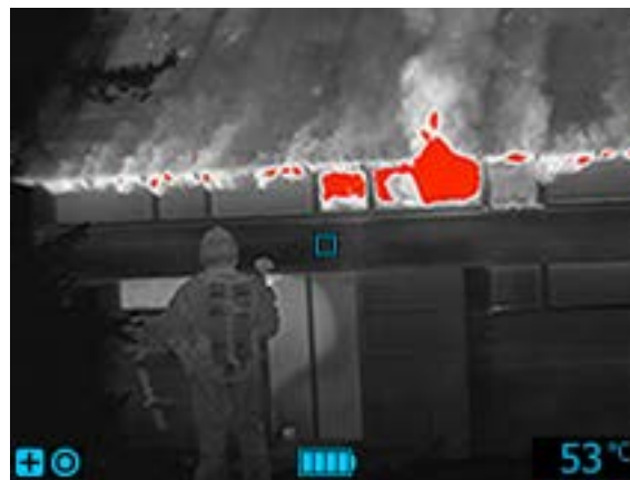
Figure 19.5 Heat detection mode.
