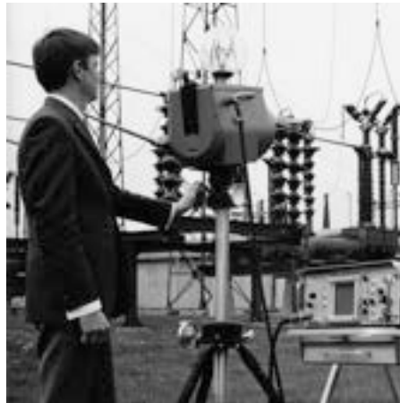
Figure 21.2 1969: Thermovision Model 661. The camera weighed approximately 25 kg (55 lb.), the oscilloscope 20 kg (44 lb.), and the tripod 15 kg (33 lb.). The operator also needed a 220 VAC generator set, and a 10 L (2.6 US gallon) jar with liquid nitrogen. To the left of the oscilloscope the Polaroid attachment (6 kg/13 lb.) can be seen.
