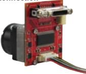
Alternately, you may use the 7-Pin PicoBlade connector. Connect it to the interface assembly as shown above. Once connected to a power source, the board will illuminate and the Boson will be active to transmit and receive signals.
