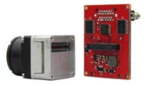
Connect the BOS-CL-SY-IF to the back of the Boson by lining up the hirose connector. Press together until you feel the board snap into place
