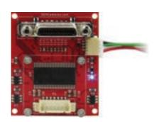
Connect the USB Cable to the Interface as shown above. Once connected, plug the USB connector into a power source or computer. The light will illuminate and the Boson will power up.
