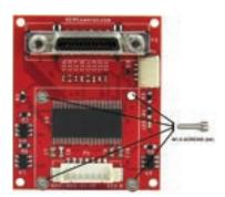
Secure the Assembly to the rear of the boson using the four cap screws provided in the kit.
