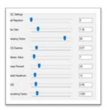
**Tail Rejection:** Determines the percentage of the histogram "tails" which
